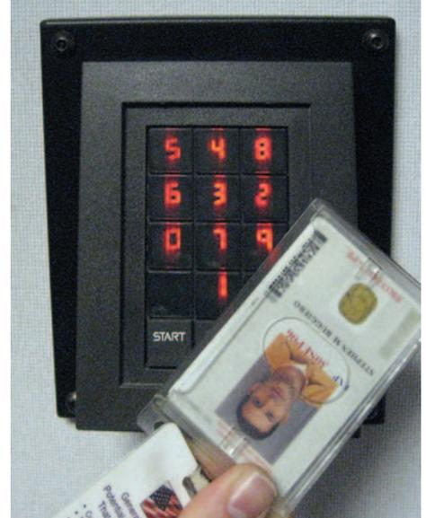
Card readers at the port include Hirsch ScrambleSmart contactless TWIC readers with high security scrambling keypads. The devices feature dual-authentication technology to verify the identity of cardholders.
